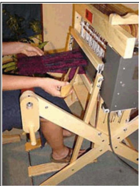
*Inserting the Shuttle*
